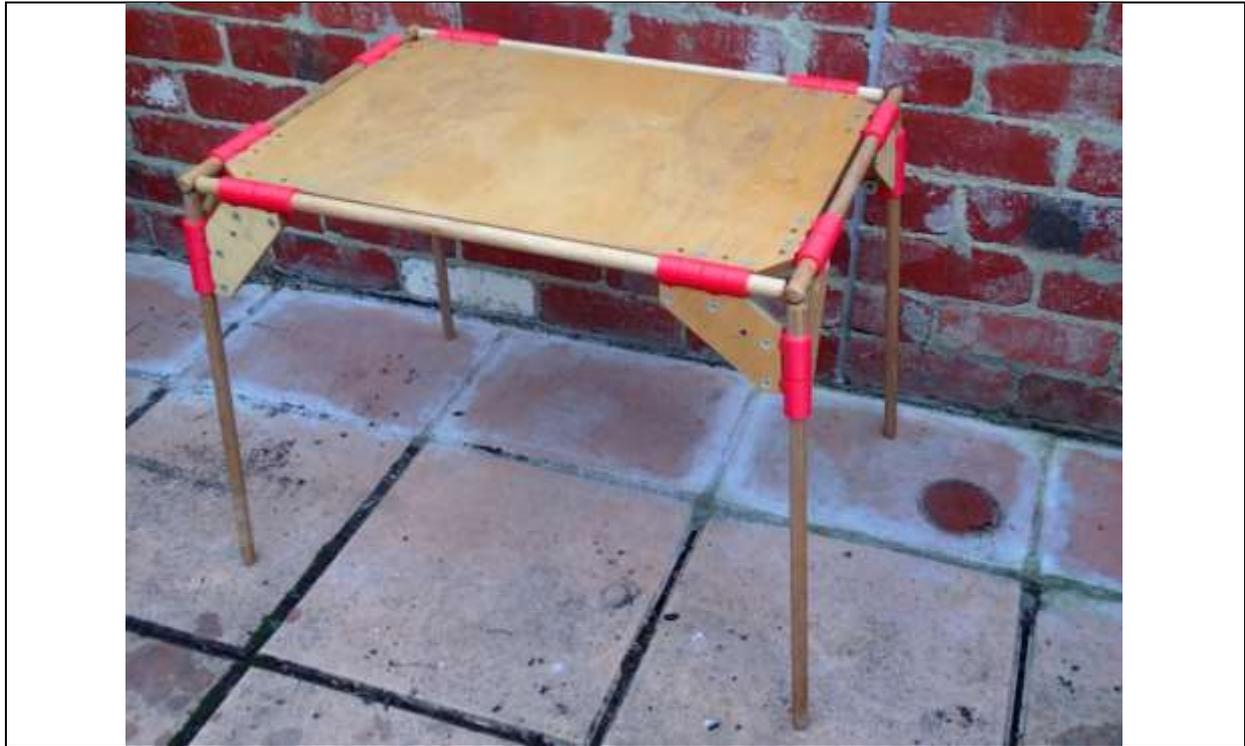
**Figure 13, Table made using 3d printed edge joins.**
